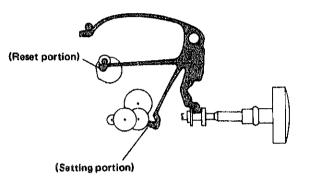
Make sure that the second setting and reset are secured by the pulling out operation of the crown.
