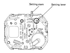
Remove the setting stem while pushing the setting lever at the site indicated by the arrow using a fine instrument like tweezers, etc. The above procedure should be carried out with the setting stem remaining in its normal position.
