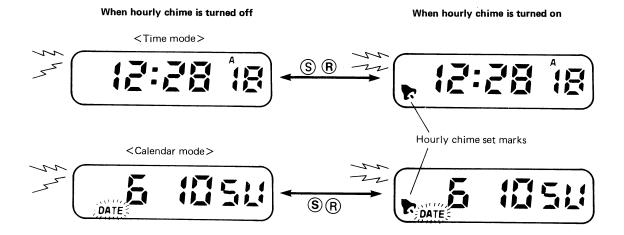
• The sound monitor is generated with a simultaneous push of the S and R buttons in the normal time mode or the calendar mode. At this moment, setting and release of hourly chime can be alternately carried out with every push of the S and R buttons at the same time.
