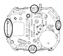
When mounting the supporter for plate complete, make sure that three points of the supporter for plate complete which are circled in the diagram have been placed within the LC display panel supporter.
