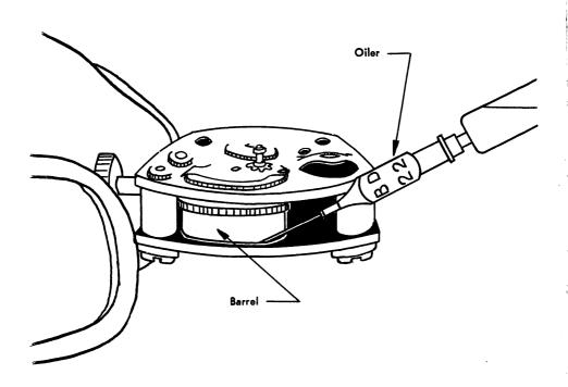
To introduce oil between the slipping tail and the inside of the barrel, hold the movement at about 45°, the barrel and front frame uppermost. Using an oiler or paddle, wipe oil into the space between the outside diameter of the barrel and the barrel sweeping in the back frame. This oil will work up between the slipping tail and the inside of the barrel.
