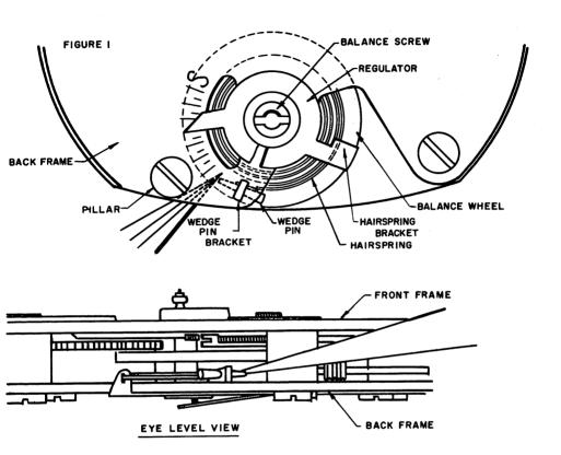
The small wedge pin holding the hairspring anchored to the bracket in the back frame should be loosened and removed. Figure 1 shows the complete operation of removal by inserting a tweezer between the front frame and the back frame, using the tubular pillar as a support for tweezers. Care should be taken as not to harm either the hairspring or balance wheel.
