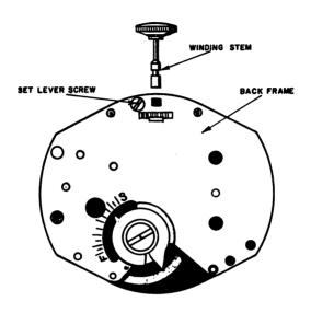
To remove the winding stem on the Model 23 movement, loosen the set lever screw, and pull the winding stem out.
