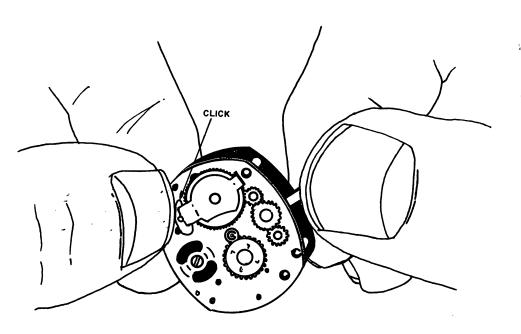
The power of the mainspring should next be released. To achieve this, the crown should be held lightly between the index finger and thumb of the right hand, while with the left thumbnail the click is released. The crown should be allowed to revolve slowly between the two fingers of the right hand until the power of the spring is completely released. Sudden release of power may do harm to the mainspring.
