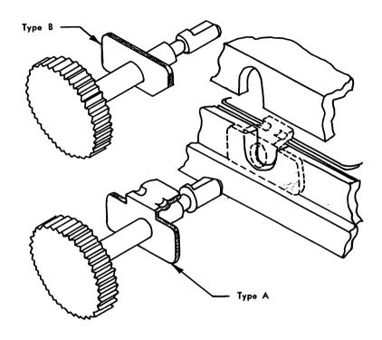
On newer non-waterproof models, the dust seals shown above are used. Type "A" is a formed metal seal with a bent tag. After being fitted to the winding stem, the bent tag should lie flat on the top face of the front frame and the body of the seal placed between the caseback and bezel. The case should then be carefully closed.
