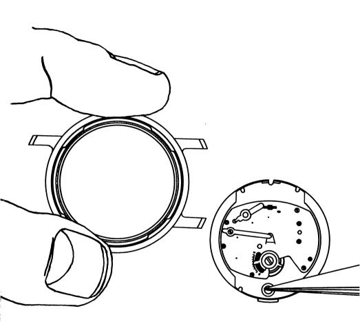
When removing the dial and movement assembly, insert the tweezers in the embossing on the dial holder.
