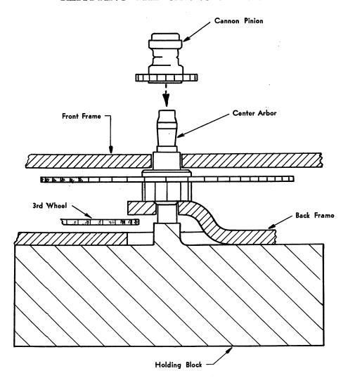
Before refitting cannon pinion a small amount of grease is applied to center arbor. The movement is then positioned on holding block so that center arbor is supported, care being taken to ensure that the center arbor is fully raised and the shoulder correctly located in the frame hole.
