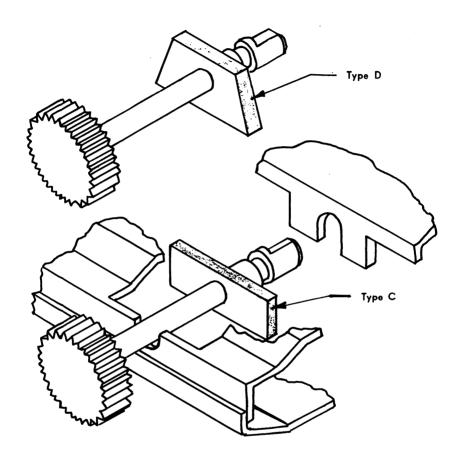
Another design of dust seal is shown here. Both types "C" and "D" are made of rubber and fit around the stem. Both seals must be located between the inside of the caseback and dial when the movement is in place prior to closing of the case. The shorter side of type "D" should lie towards the dial side of the movement.
