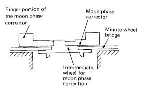
(3) Lightly press the axle head of the intermediate wheel for moon phase correction with a tip of tweezers.
