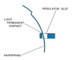
Inspect the hairspring to be certain that it is properly adjusted. As shown by the diagram, the hairspring should be in light, permanent contact with the inside edge of the regulator slot. The hairspring should not leave the inside edge of the regulator slot at any time during the complete maximum occilitation of the balance.
