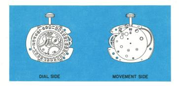
The Timex Model 25 is an  $11\,\%$  " x  $9\,\%$ " calendar movement utilizing the basic construction of the Model 24. Like the Model 24 it features a "V-Conic" Bearing system and rugged two plate design. The entire Calendar mechanism is efficiently housed between the dial plate and dial.
