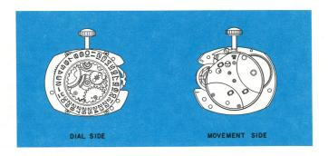
The Timex Model 75 is an 11-1/4 ligne by 9-1/4 ligne, 21 jewel calendar movement featuring rugged two plate construction. The Model 75 is readily distinguished from other Timex movements by the number of jewels and the small, gracefully decorated movement plate.
