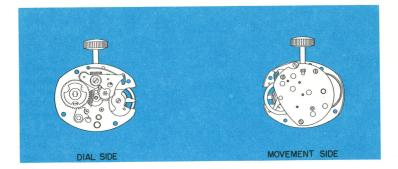
The TIMEX Model 78 is an  $8^{\prime\prime\prime} \times 9^{1/2}^{\prime\prime\prime}$  movement featuring ''V-conic'' bearings system and rugged two plate design.
