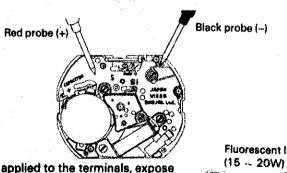
(2) With the probes applied to the terminals, expose the solar cell to a light from a flourescent lamp (15 to 20W) 5 cm directly above the watch.
