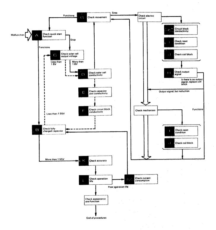
(4) Procedures for checking and adjustment
