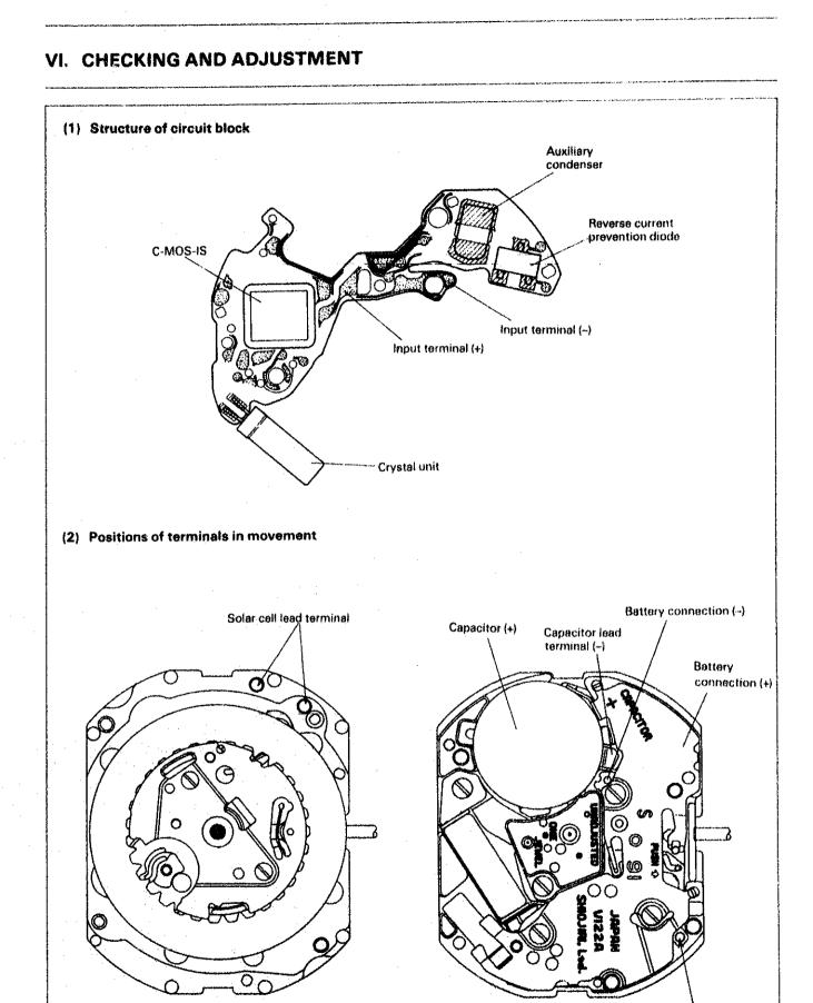
Solar cell output voltage measurement terminal
