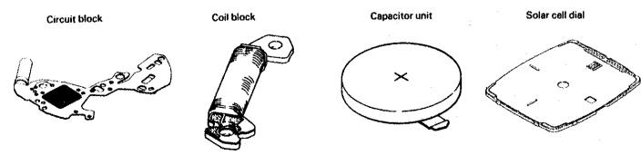
Be sure to clean only stains on the conductive portions of the circuit block, etc. with a cloth moistened with benzine,
