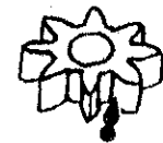
The teeth of the intermediate wheel for calendar correction
